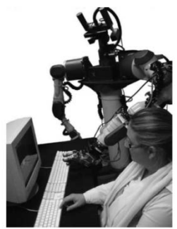
Figure 1. Experimental setup: Social Simon task shared between a human and a humanoid robot.
